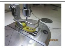
No.2 Corrective action taken – needle guard equipped
